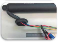
3. Cut the wiring harness of the replacement drive about 5cm (2 inches) behind the grommet. The separated remainder of the wiring harness of the replacement drive is no longer needed.
